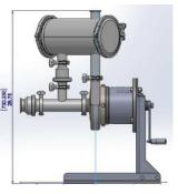
This accesorie is special designed for any QC and QIS series pump to convert them in a self priming pump ideal for handling air, upto 60%, principally used as CIP return pump.
